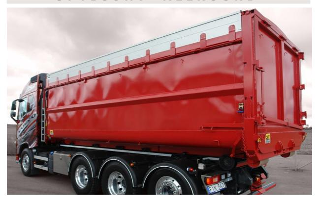
Allround is the right name for this Opticont model. demolition, waste, wood chips, scrap or grain. With the Opticont Allround, the same container can be used for many different kinds of haulage.
